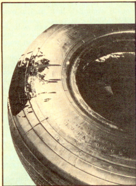
Oil, tar, brake fluid, degreasing agents and chemicals can cause rubber to deteriorate. Tires should be wiped clean with a gasoline-dampened cloth and then washed immediately with soap and water.
